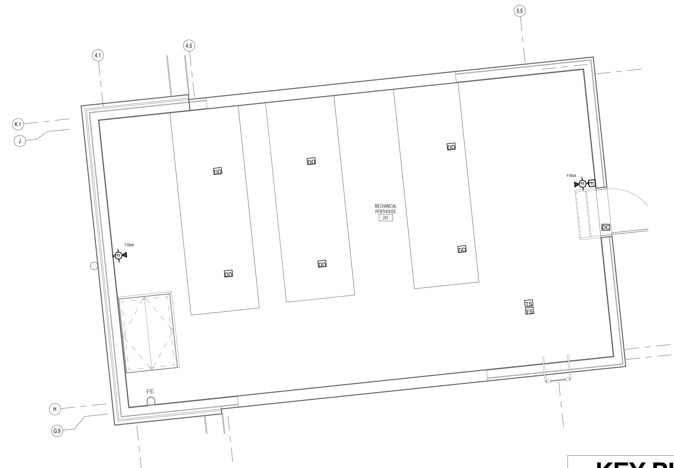
PART PLAN - PENTHOUSE - FIRE ALARM & SECURITY 1/4" = 1'-0"
